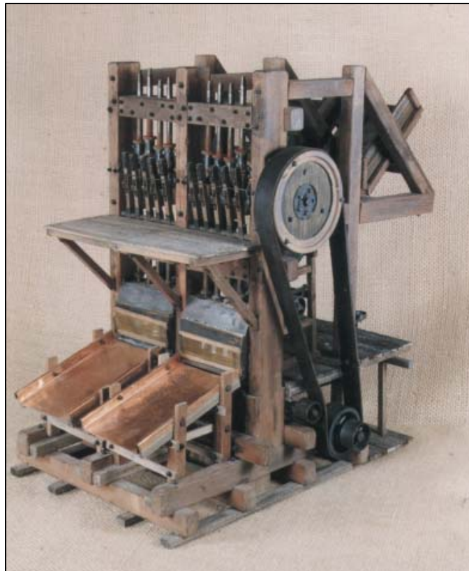
Miniature replica of a stamp mill crusher similar to that used throughout the gold districts of Nova Scotia.
